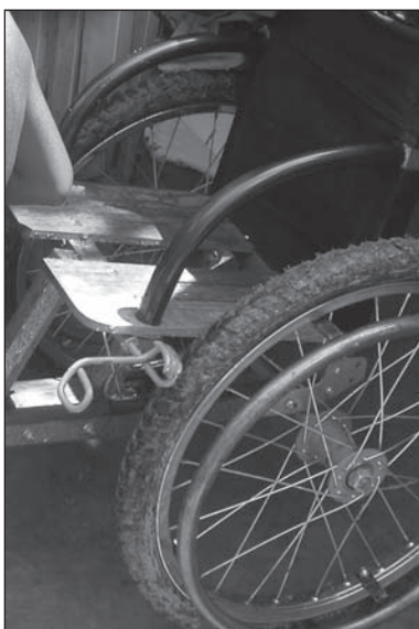
Figure 9.75. Wheelchair seat with central plank removed.
