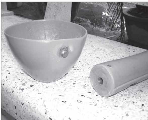
Figure 6.77. Screw attachment on a bowl for an artificial arm.
