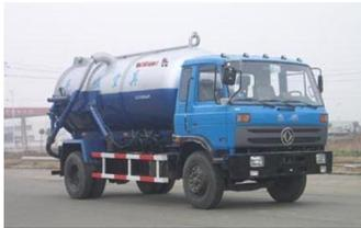
The conventional method for pit emptying is the vacuum tanker. This is a truck-mounted tank between 1 to 10 m<sup>3</sup> in with a vacuum pump connected to the tank to suck out the sludge commonly used in industrialised countries. However, there are technical limitations to the use of the vacuum tanker in areas with inadequate road access, shortage of spare parts and fuel.
