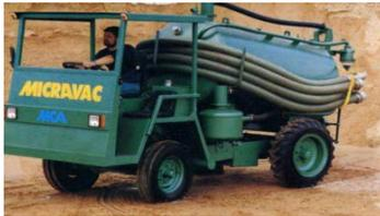
The Micravac is a micro vacuum tanker developed for use on uneven roads and areas with poor access.
