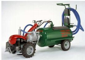
The Dung Beetle is a machine developed by a Dutch company J.Hvidtved Larsen and deployed in Ghana. This machine uses a two wheel tractor based drive, with the driver sitting on the tank and steering using the long handles on the machine. These machines have been successfully used for many years in Ghana. Useful specifications of the machine are:
