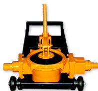
The diaphragm pump is manually operated for emptying the wet pit latrines. The sludge is pumped into a bucket or small drums. The pump cannot be produced locally. Like the gulper a grid or mesh is placed at the intake of the pump to prevent large items to enter the pump. The pump can only empty wet latrines (sludge that is liquid). The cost for pump and hoses is estimated to be around 300 USD.
