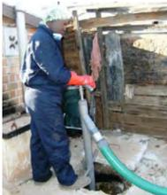
A relatively new technology type in the Manual Pit Emptying Technology (MAPET) category, is the London School of Hygiene and Tropical Medicine (LSHTM) Sludge Gulper. This is a hand pump that can be lowered into a pit or tank and used to lift the contents out into a bucket. The system is currently still being trialled on varying types of sludge. Whether it performs successfully in all locations is yet to be seen.
