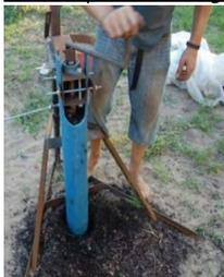
The Pit screw auger is designed for solid sludge, such as the sludge found in open pits. It uses an auger and its flow ranges from 7 L to 20 L per minute.
