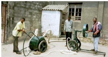
This MAPET system comprises a hand-pump connected to a vacuum tank mounted on a pushcart. A hose connected to the tank is used to suck sludge from a pit or a septic tank. When the hand pump is turned, air is sucked out of the vacuum tank and sludge is sucked up into the tank. Depending on sludge consistency, this product can pump the sludge from a maximal depth of 3 m.
