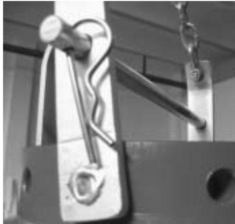
2.- Ensure that the safety ring has been correctly adapted
