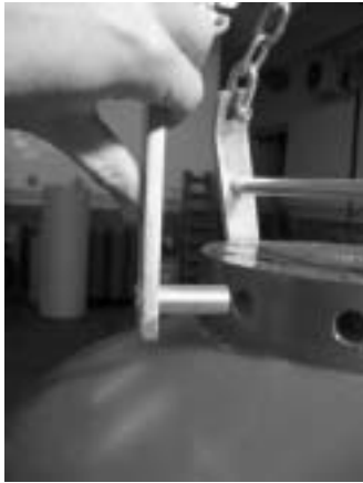
1.- Introduce the four metallic pins into the holes of bolts.
