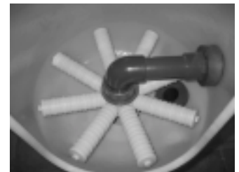
5.- Glue the piping necessary to adapt accessories and screw required arms to the distributor to complete the distribution system.
