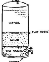
Keep the filter covered and full of water (up to 2-3 cm from the top). When after 2-4 weeks the water starts to flow slowly the filter needs cleaning. Clean the filter by scraping off the top layer of sand. After four or five cleanings you will need to add more sand. To do this you will need to drain out the water until the water level is 10 cm below the level of the sand.
