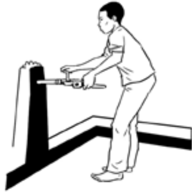
2. Open upper biptap assembly using a 14" pipe wrench.
