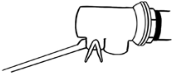
1. The faulty float valve.
