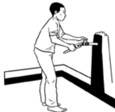
6. Replace the assembly, open supply of water to tap, check to confirm no leaks.
