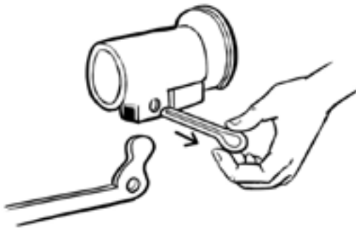
3. Remove the lock, thus releasing the connecting rod to the ball valve.
