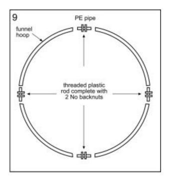
the correct position in a corrugation has been located, the backnuts should be screwed in opposite directions to expand the hoop firmly into a corrugation. This will have the effect of tightening the funnel even more.
