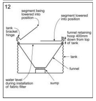
13. On each of the six tank assembly brackets, rotate the crosspiece to lock the segments in place. Assemble the central beam member by attaching the central dish support arm to it and lower this into place, making sure the central dish covers the ends of the segments and bolt the central beam onto the two tank bracket hinge assemblies. This assembly will help prevent the segments lifting in the centre of the tank when the system is in operation.
