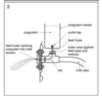
the Tee and into the incoming water flow and coagulant introduced at a constant rate.
