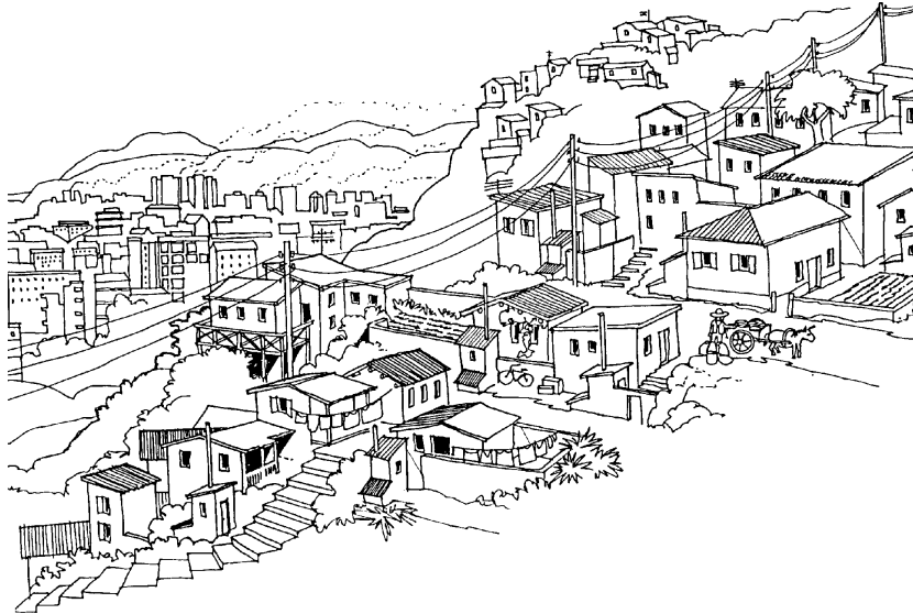
Figure 5.2 A neighbourhood with an ecological sanitation system. Each household has its own dehydrating or composting toilet attached to the house. There is urine diversion and the processing chamber is solar heated. Municipal workers collect urine, primary processed faeces and kitchen wastes and take them to the neighbourhood's own recycling station.
