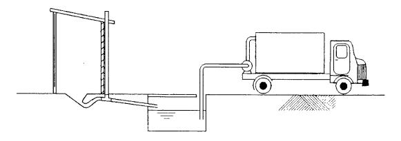
Figure 3. Vault latrine being pumped out by tanker
