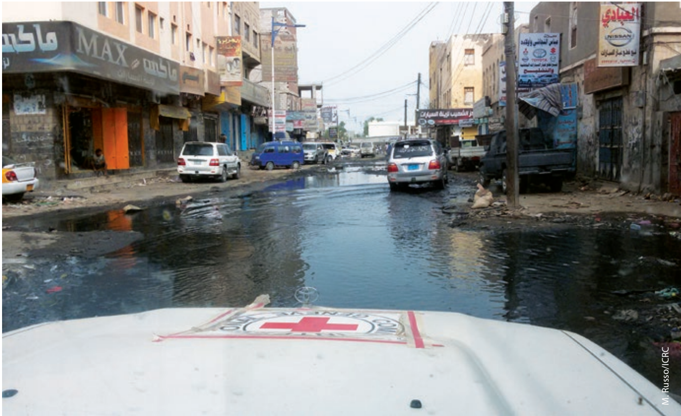
Photo 6. Interconnectivity between essential services needs to be understood and properly integrated into an emergency response to a breakdown in order to avoid counterproductive effects. Retrofitting the broken water supply network to this quarter without addressing the damaged sewage evacuation network would increase the exposure of the population to public health risks by causing sewage to spill over into the streets. (Aden, 2015)
