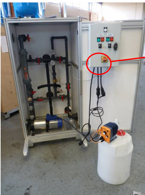
Assembled control panel ready for use
